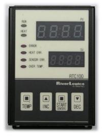
✓ PV : Display for Present Value of a temperature sensor
